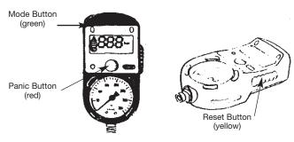
The RESET/OFF yellow button resets the device from the full alarm mode. It also shuts the unit off after the cylinder valve is closed and all air pressure is bled from the unit. The center red (alarm) button activates the full alarm mode with or without air pressure.
