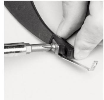
2. Use a Phillips screwdriver to unscrew the lower clip screw.
