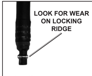
FIGURE 5 Inspecting Male Quick Disconnects
