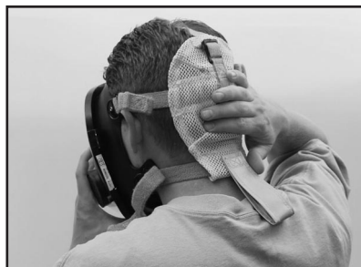
FIGURE 13H HEAD HARNESS MUST BE FLAT
