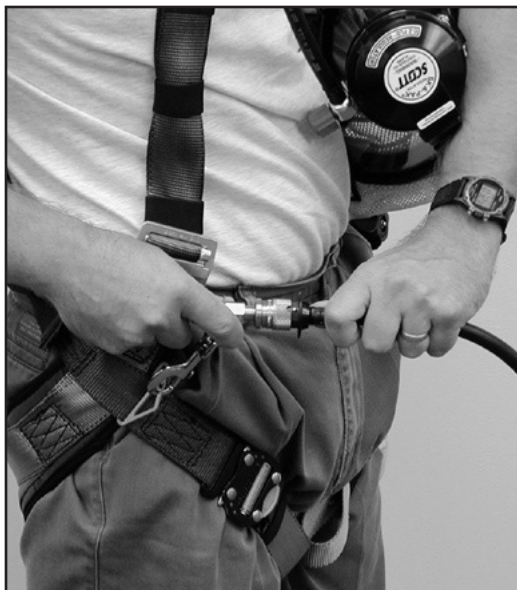
FULL BODY/FALL PROTECTION HARNESS CONNECTING SUPPLY HOSE AND "STANDBY" CONDITION
