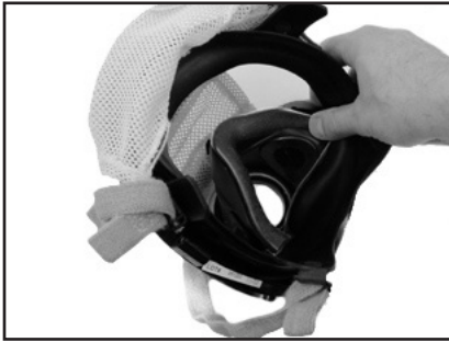
FIGURE 9 Checking Voicemitter Ducts
