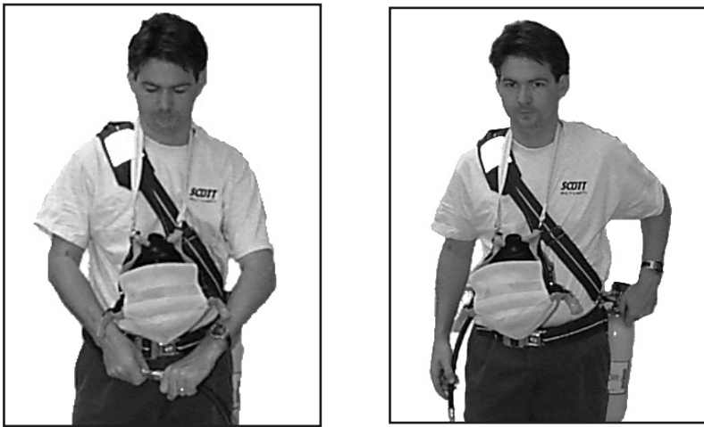
CONNECTING SUPPLY HOSE AND "STANDBY" CONDITION (SKA-PAK PLUS SHOWN WITH OPTIONAL NECK STRAP ASSEMBLY)
