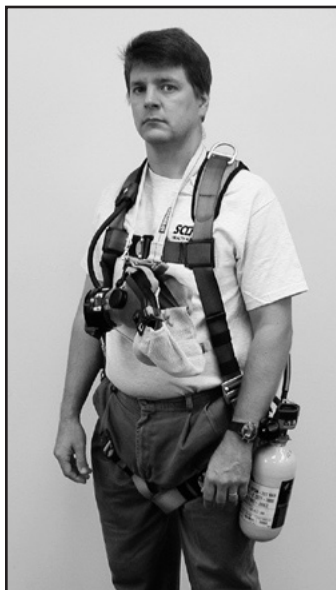
FULL BODY/FALL PROTECTION HARNESS CONNECTING SUPPLY HOSE AND "STANDBY" CONDITION
