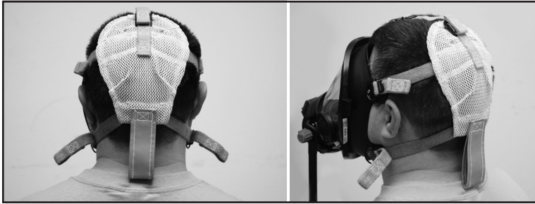
CENTER HEAD HARNESS ON THE CROWN OF THE HEAD FIGURE 20-I
